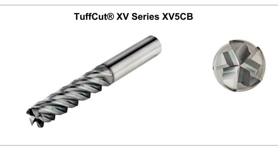
The M.A. Ford® XV5CB is a stable, reliable solution for deep, dynamic milling applications. This 5 flute chipbreaker end mill is designed to deliver exceptional metal removal on steels and stainless steels. Offered in both 3xD and 4xD length of cut options and diameters from 3/8" to 3/4". The XV5CB increases productivity by utilizing its aggressive stepover capabilities.
